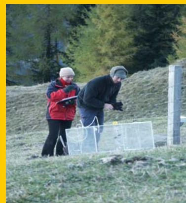
Figure 1: Portable, closed-dynamic ecosystem chamber for measuring NEE in complex terrain.
