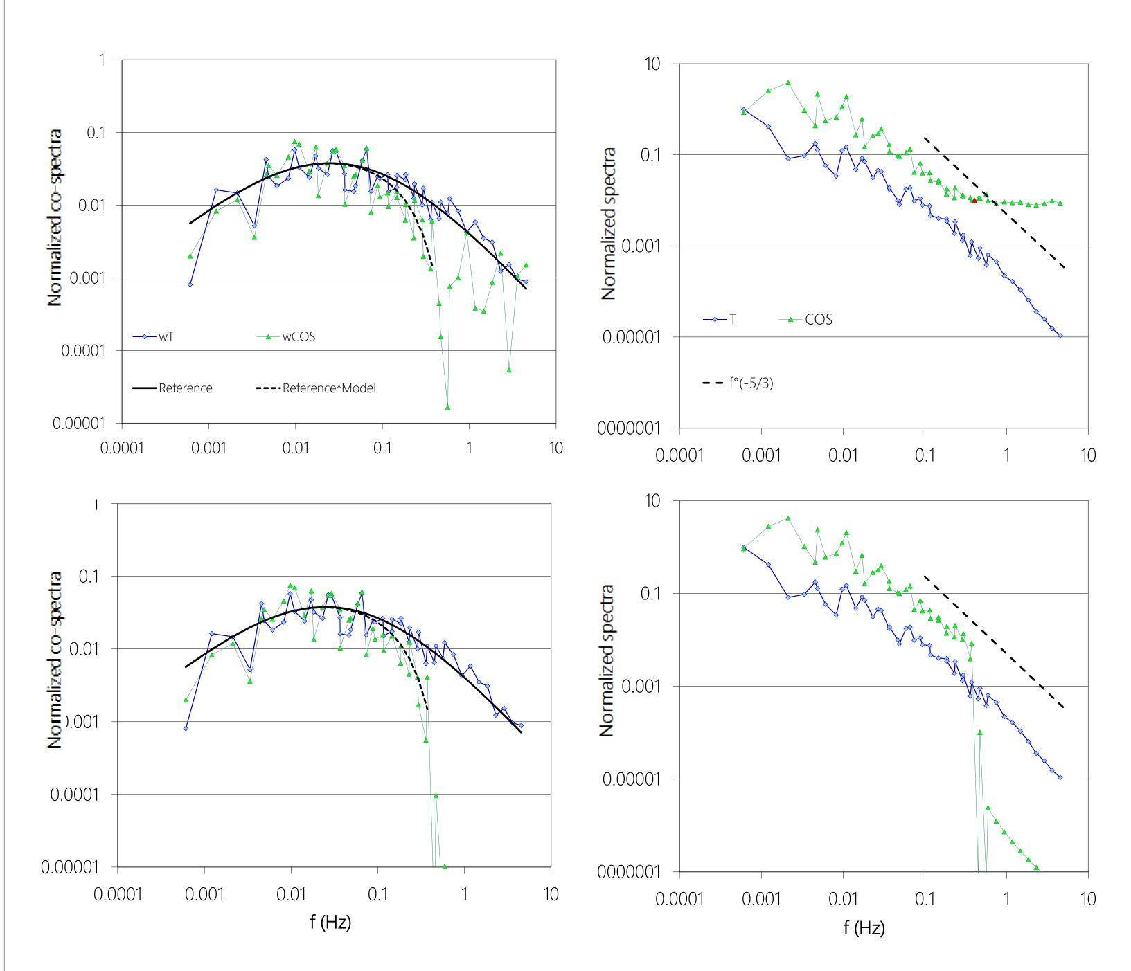
Fig. 3: Co-spectra (left panels) and power spectra (right panels) before (upper panels) and after (lower panels) application of the FIR filter. The onset of QCLAS noise is indicated by a red triangle. Solid and dashed lines in the cospectral plots indicate the reference model and the attenuated reference model, the integrated ratio of which yields the low-pass filtering correction factor (x in this case).
