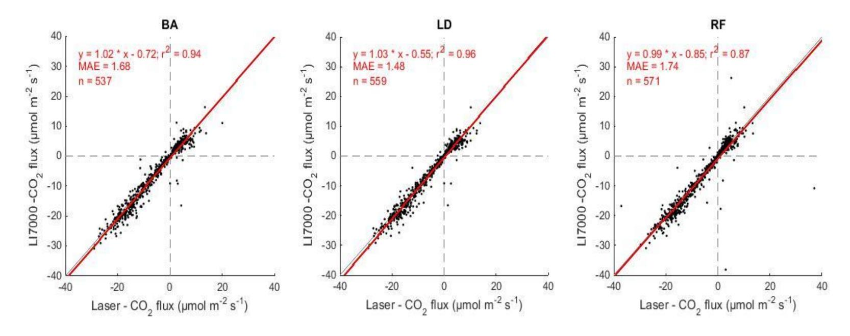
**Fig. 4:** Correlation between IRGA (Li-7000) and QCLAS  $CO_2$  fluxes using block averaging (left panel), linear detrending (middle panel) and a recursive filter with a 50 s time constant (right panel).
