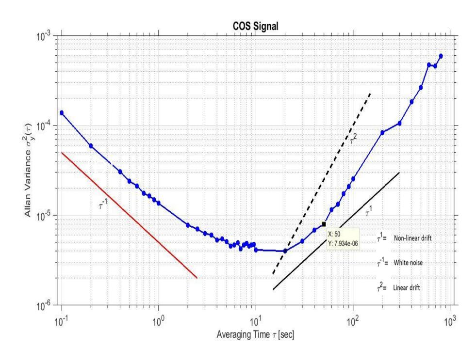
Fig. 2: Example Allan variance plot for COS. The time series was obtained under ambient conditions in the instrument hut in the field by feeding pressurized air from a cylinder to the QCLAS.
