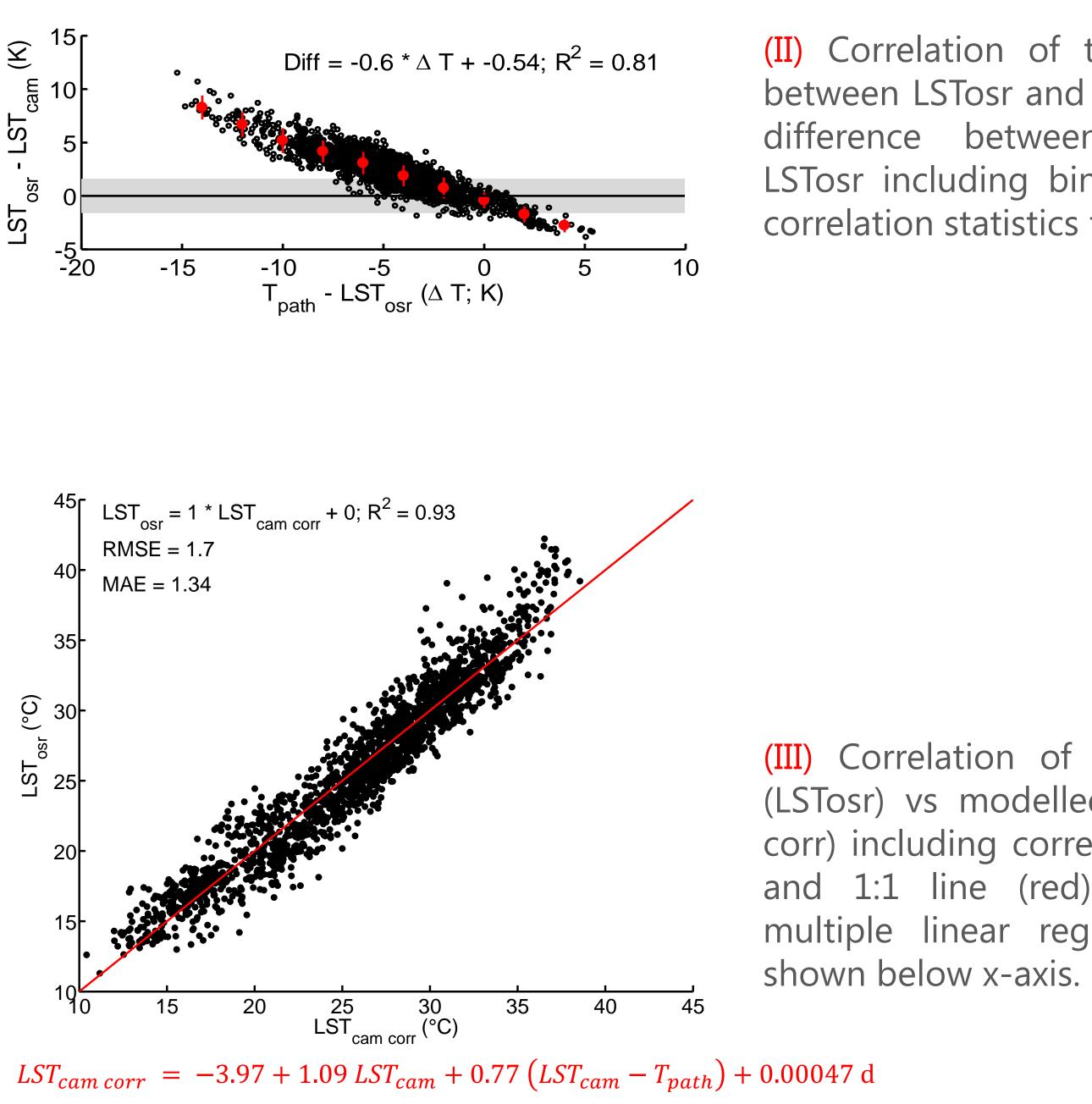
(II) Correlation of the differences between LSTosr and LSTcam vs. the difference between Tpath and LSTosr including bin-averages and correlation statistics for raw data.
