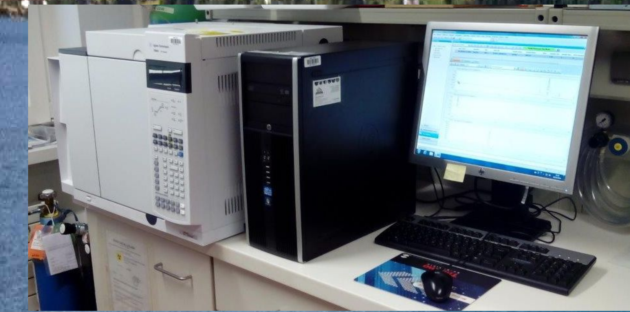
Fig. 3: Gas Chromatographer equipped with Flame Ionization Detector for CH 4 analysis.
