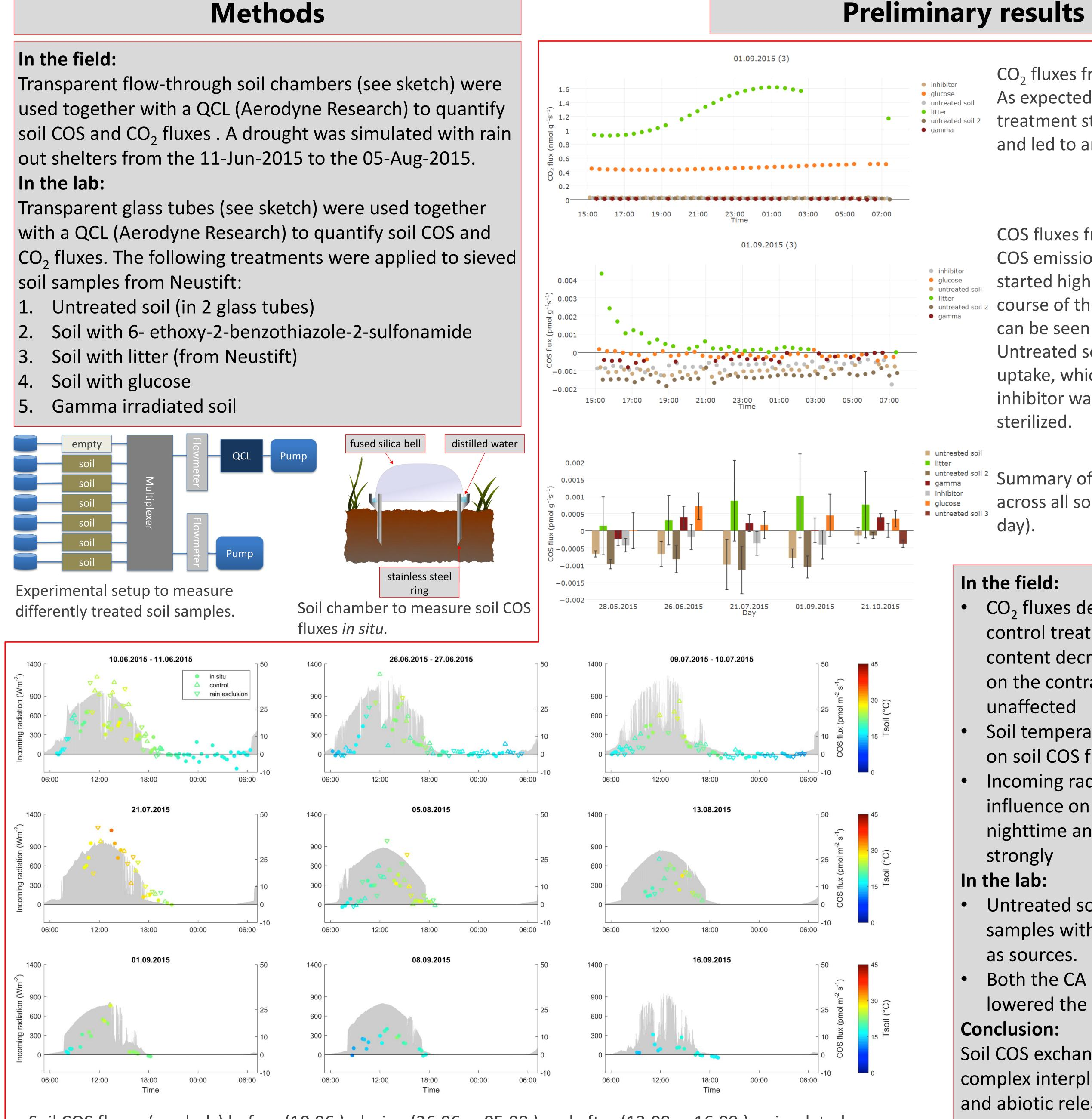
Soil COS fluxes (symbols) before (10.06.), during (26.06. – 05.08.) and after (13.08. – 16.09.) a simulated drought. Grey bars indicate the incoming solar radiation.
