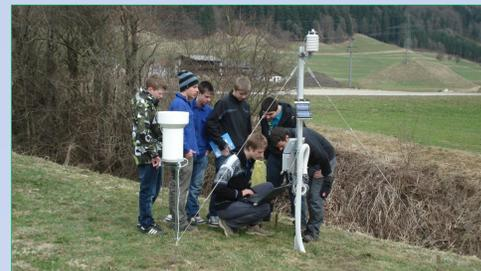
Pic. 2: Young farmers study the function of the micrometeorological station at one of the ten study sites. Measured variables are photosynthetically active radiation (PAR), precipitation, air and soil temperature, humidity, and soil water content.
