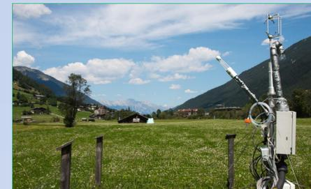
Pic.3: Eddy covariance flux tower in Neustift in the Stubai valley. The measured CO<sub>2</sub> net ecosystem exchange is used for calibrating the GrassC model.
