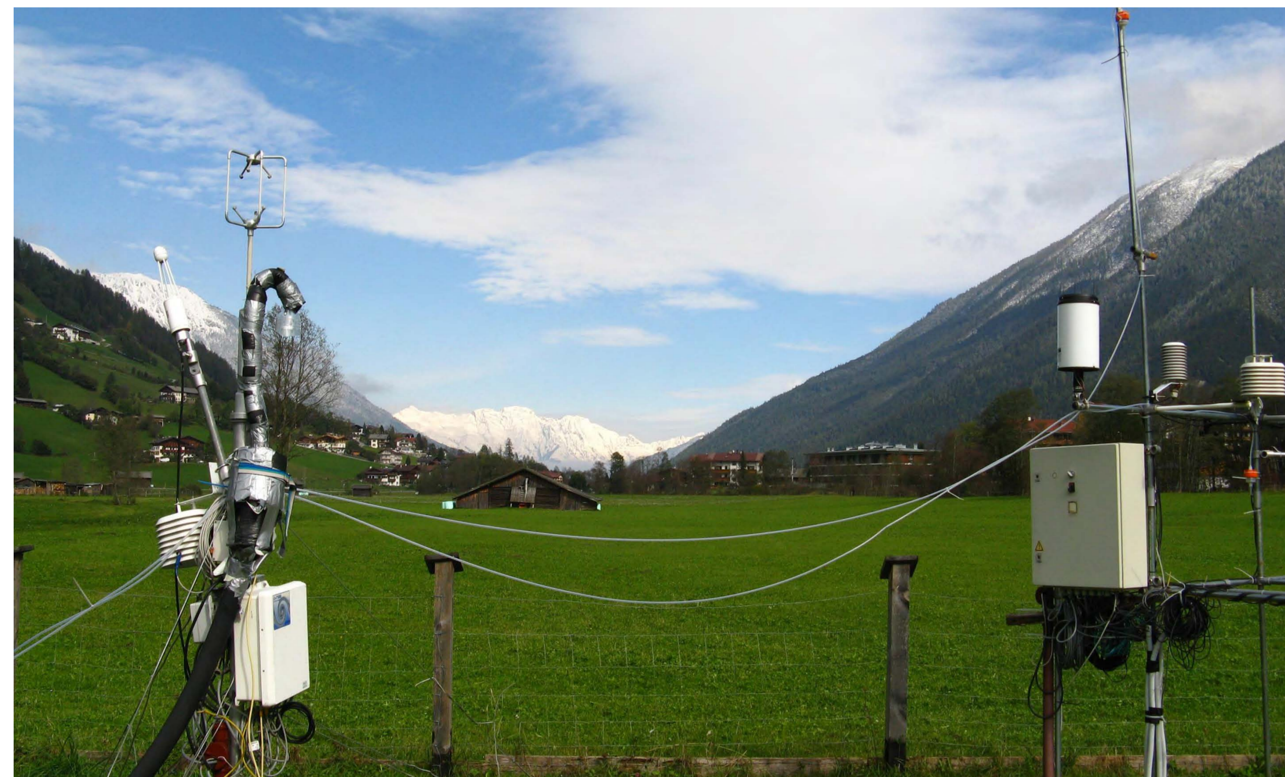
Figure 1: Measuring system at the field site in Neustift. To the left the gas inlet for the PTR-MS and the sonic anemometer and to the right the automated weather station.
