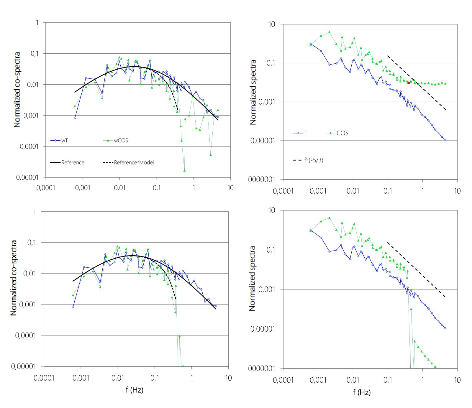
Fig. 3: Co-spectra (left panels) and power spectra (right panels) before (upper panels) and after (lower panels) application of the FIR filter. The onset of QCLAS noise is indicated by a red triangle. Solid and dashed lines in the cospectral plots indicate the reference model and the attenuated reference model, the integrated ratio of which yields the low-pass filtering correction factor (1.15 in this case).
